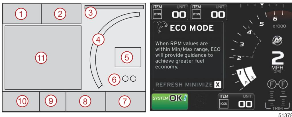
1. Volts or Depth: This data box is user definable. A list of the available data parameters can be modified in the Settings menu.
