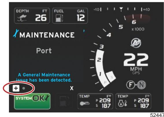
2. Open the + icon to expand the text. You can reset the maintenance to 100% or exit the screen.
