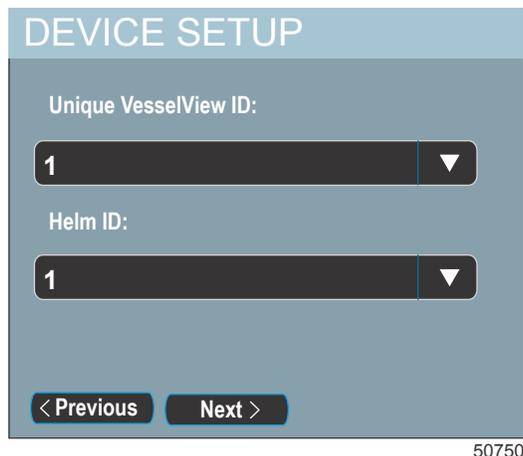
2. Press the enter button to open the Unique VesselView ID option. Use the arrow button to highlight the ID number and press enter. Choose a number that is different from the other numbers assigned to any other VesselView unit installed.
