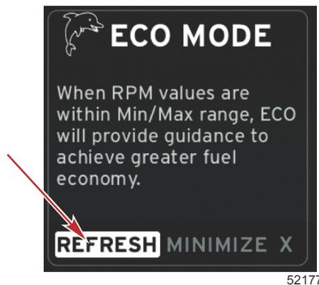
3. When the system has finished calculating new targets, the contextual data area will change to indicated the values have been refreshed.
