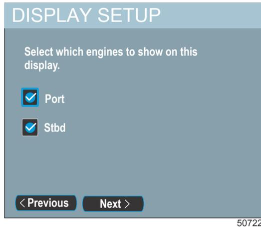
2. Press the arrow button to highlight which engine is to be displayed, and press enter. The following is a description of what may be available, depending on the number of engines:
